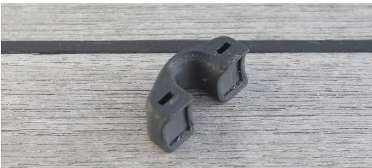
The extrusions at the "feet" can be carefully filled with an elastomer of choice (such as Sika or Butyl tape) to improve grip on the stanchion.
