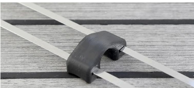
Standard 5mm wide stainless steel cable ties are threaded into the cut outs of the fitting. When tightening the cable ties, push back the locking ball with a small flat-head screw driver to achieve a tight fit.
